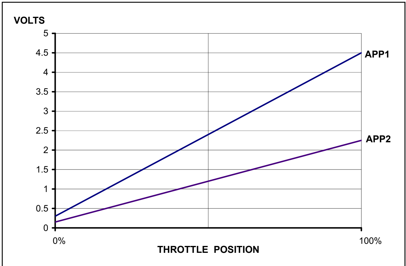
Figure 63 APP Sensor Signal (Approximate Values)
