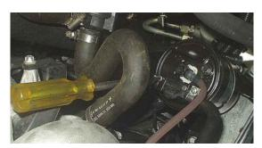
twist the fitting). This return line does double duty. In the block with the fuel return lines is a bimetal valve that directs the returned and warmed fuel into the filter when it is cold (below 80 degrees F), or back to the tank when the filter is warm (over 80 degrees F). The picture here was taken on reassembly, so the line to the pump (step 4 above) is already in place.
