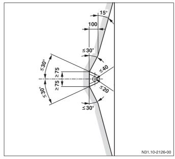
Open-jaw coupling, top view
