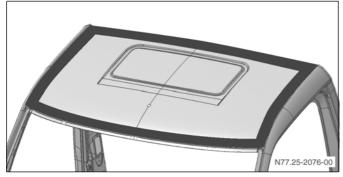
Adhesive for fitting wind deflectors should be applied in the area shown
