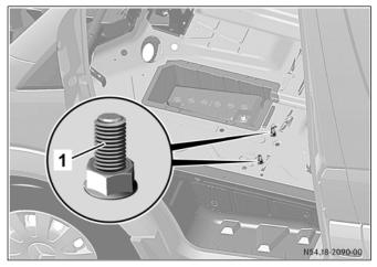
Cab earth connection, co-driver's seat bodyshell
