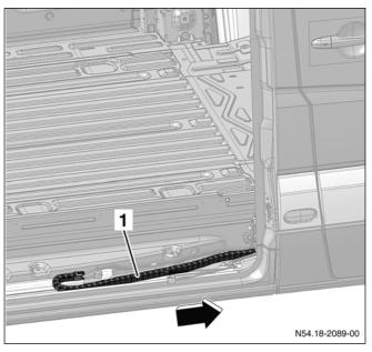
Load compartment sliding door with energy chain
