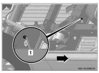
Frame earth connection (3.5 t to the front of the rear axle)
