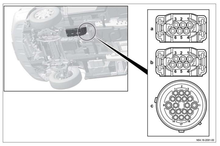
Position of low frame interface connector behind battery box
