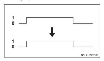
► Button: the signal in the signal pool is toggled with each 0 -> 1 switch of the input.
