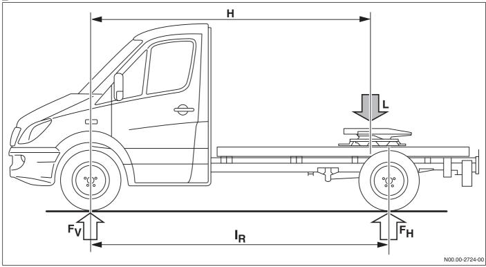
To avoid exceeding the maximum axle load, the position of the semitrailer coupling is calculated as follows:
