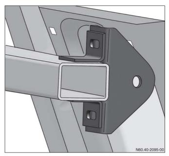
Connecting the longitudinal tube to the support
