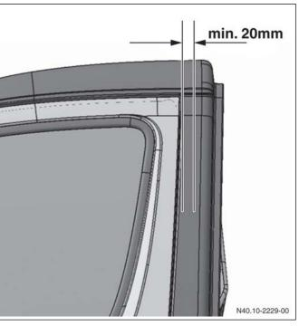
Minimum distance between rear edge of door and integrated body
