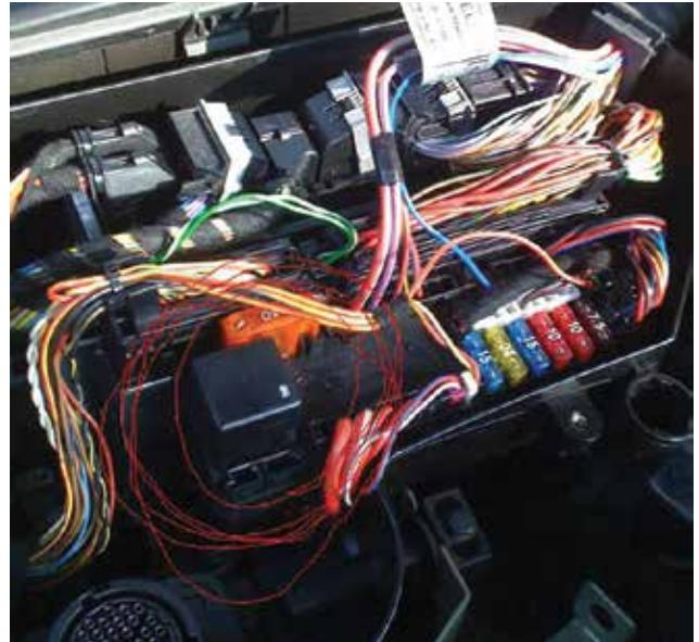
*These days pulling fuses one at a time while watching the milliamp draw reading taken between the negative battery post and the cable clamp is "Verboten." Instead, read the mV drop across the fuse, then convert that to mA.*
