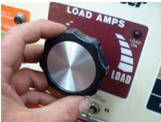
*Although Mercedes-Benz recommends the use of the sophisticated battery testers from Midtronics, some technicians still like to double-check real-world capacity with an old-fashioned VAT and its carbon-pile load.*
