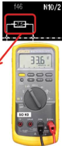
The voltage drop across a fuse, minus the known nominal resistance for a fuse of that amperage, will yield the actual current draw in mV, which can then be converted to a more helpful reading in mA.
