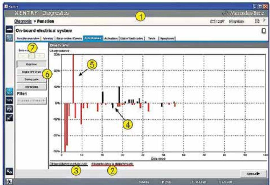
XENTRY screen with all driving and engine OFF cycles.
