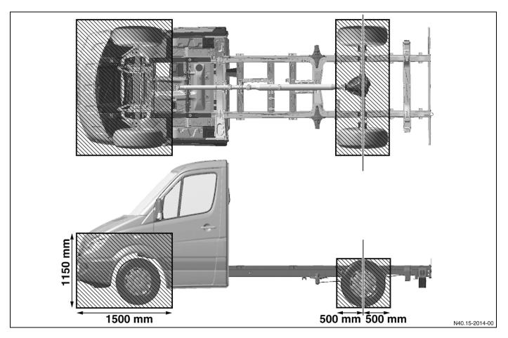
Restricted area for tire pressure monitoring system. TPMS only available on 2500 SPRINTERs. Picture above reflects 2500 SPRINTER Chassis-Cab for illustration purposes only.
