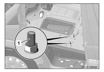
Cab ground connection (inside driver's seat base) 1 ground bolt connection
