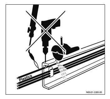
Test each of the systems for pressure loss and leaks after installing compressed-air lines and hydraulic lines. No other lines may be attached to brake hoses. Lines must be protected from heat by means of insulation.
