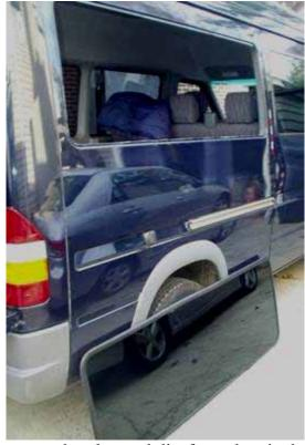
Remove the glue and dirt from the pinch weld flange.
