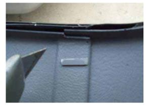
The new window's compression strip goes over the plastic. There is no gasket on the inside to fill in any gaps. Therefore, reduce the bumps by trimming the four places around the window that the plastic overlaps. Install the supplied foam gasket to the inside of the frame on the window. Do not remove the film protecting the glue until first testing the location of the window.
