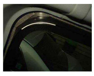
This is how the corners look with the window properly shimmed. The exterior aluminum frame covers the skin of the van. There are no gaps between the window and the skin of the van.
