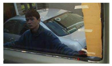
When the gasket has been relocated along the full bottom and some of the lower radius of the window, position someone on the outside to help pull the window out and catch it if it decides to fall out while the inside person works on the gasket.
