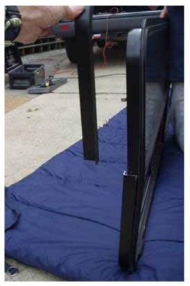
A step back: The instructions provided by Peninsula show a diagram on how to apply the compression frame. However, the diagram is incorrect, as it shows a "S"- frame with the outer flange extending away from the window to accommodate a thick wall. The "S" flange for the pinch-weld window must go under the window to reach the wall of the van.
