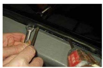
Start pushing the lip of the gasket over the pinch weld.
