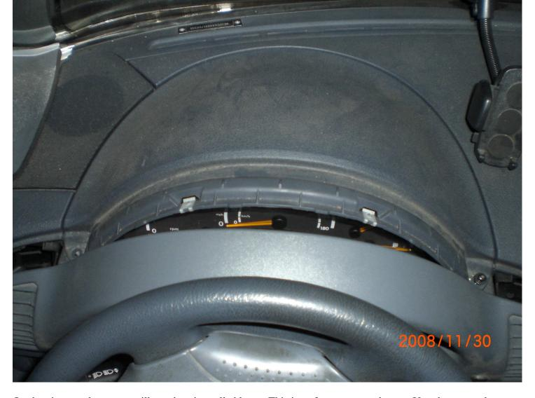
On the pictures above you will see the trim pulled loose. This is as far as you need to go. You do not need to completely remove it or disconnect the wires to the optional switches. This will expose 2 more #20 Torx screws on either side of the dash cover over the top of the cluster. After removing them, remove the cover.
