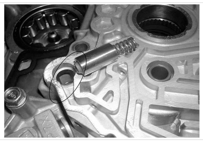
Loss of TCC or TCC slip: Created by end plug loose at the TCC control valve. A cross leak of converter charge oil into TCC control negatively affects TCC control. Inspect the stator for cross leakage at the finished area, where it passes through the casting.
