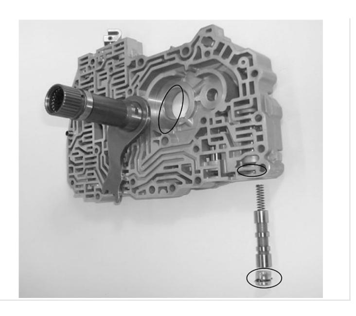
**2.** Restricted coolers create back pressure on the hydraulics and either slow the stroke of the valve or cause it to stop midstroke.
