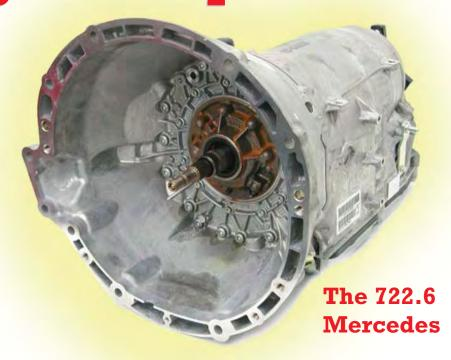
Once you've removed the valve body and bellhousing bolts, the case just lifts off the entire gear train assembly (figures 1 and 2). This makes for easy gear train disassembly and reassembly.
