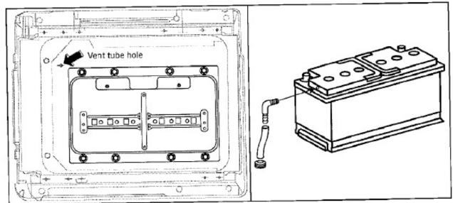
Fig 5, Battery vent tube setup
