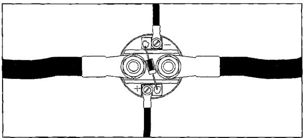
Fig 12, Isolation relay wiring
