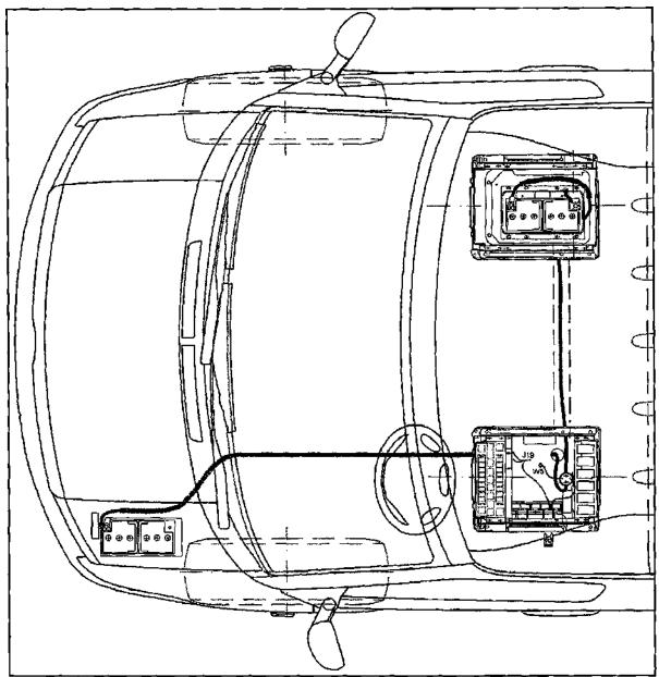
Fig 10, Auxiliary battery wiring layout
