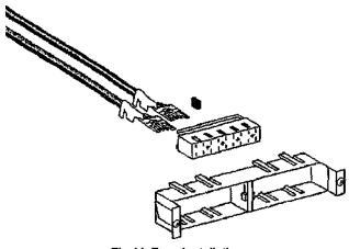
Fig 11, Fuse installation
