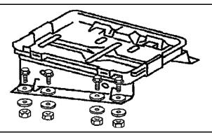
Fig 4, Battery tray installation
