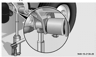
The vehicle jacking point is locked next to the front recess for the leaf spring.
