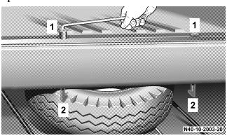
Retaining screws for the spare wheel structural member (1)
