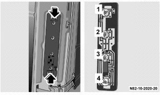
Brake lamp, taillamp, standing lamp, P21/5W – 12V 21/5W
