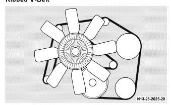
The ribbed V-belt drives the accessories, such as generator, coolant pump and hydraulic steering pump.
