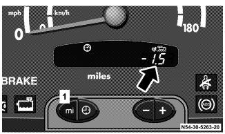
If the engine has reached normal operating temperature, the engine oil level can be displayed on the multi-function indicator for about 5 minutes after the engine has been switched off.
