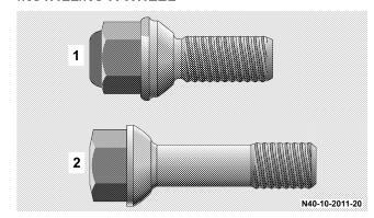
Wheel bolts for pressed steel wheels (1) Wheel bolts for light-alloy wheels (Optional) (2)
