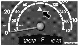
When the key is in position 2 in the ignition lock, the warning lamp in the speedometer will light up for about 2 seconds. It must go out when the engine is running.
