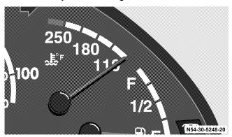
The coolant temperature is displayed when the key is in position 2 in the ignition lock.
