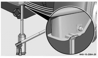
The vehicle jacking point is located under the longitudinal member in front of the rear axle.
