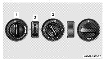
In preheat mode, the blower is automatically switched on at blower speed 1 when the water heater is switched on. When driving, the airflow control switch (2) can be set as desired.
