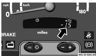
If the indicator lamp lights up briefly when the engine is running, the engine oil level has dropped to the minimum mark. Check the engine oil level without delay and add oil to the upper mark on the dipstick.
