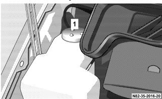
1. Washer system fluid reservoir When topping off, add windshield washer fluid ("S" for summer or "W" for winter) to the water.
