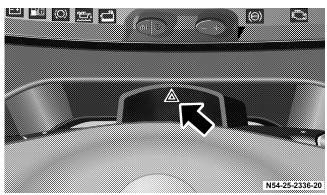
The switch is located on top of the steering column housing.
