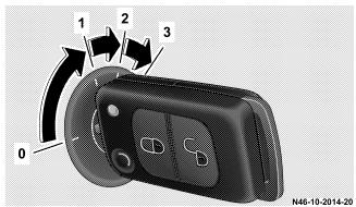
O The steering wheel is locked when the key is removed
