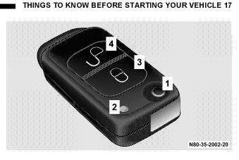
Release button for mechanical key (1)
