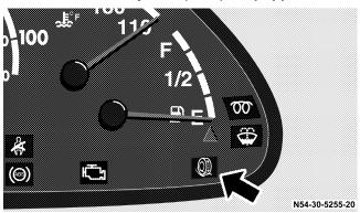
When the key is in position 2 in the ignition lock, the indicator lamp will light up in the instrument cluster as a function check. It goes out when the engine is running.
