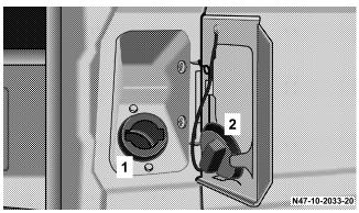
The fuel filler neck (1) is located behind the fuel filler flap next to the driver's door. The fuel filler flap can be opened when the driver's door is open. Turn the fuel filler cap (2) on the fuel filler neck (1) counterclockwise and take it off. For cargo/passenger vans, place the fuel filler cap (2) in the holder on the inside of the fuel filler flap.
