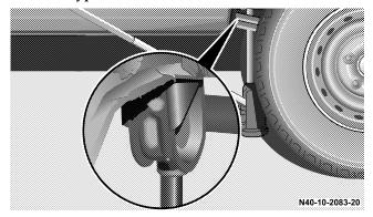
The vehicle jacking point is located under the longitudinal member in front of the rear axle.
