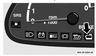
When the key is turned to position 2 in the ignition lock, the coolant level indicator lamp / in the instrument cluster lights up for about 2 seconds. It must go out when the engine is running.
