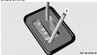
In the case of power failure the transmission selector lever can be manually unlocked (for vehicle towing).
