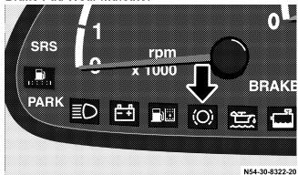
When the key is turned to position 2 in the ignition lock, the indicator lamp in the instrument cluster lights up for about 2 seconds. It must go out when the engine is running.
