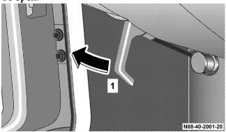
1. Pull the release lever (1). The hood then opens slightly and is restrained by the safety catch.
