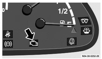
When the key is in position 2 in the ignition lock, the engine control unit indicator lamp will light up in the instrument cluster. It must go out when the engine is running.
