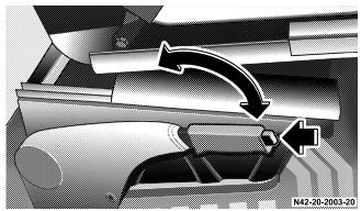
Only apply the parking brake when the vehicle is stationary.
