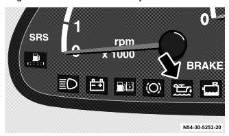
The engine oil level indicator lamp lights up in the instrument cluster when the key is turned to position 2 in the ignition lock. It must go out when the engine is running.
