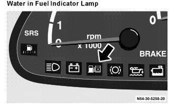
When the key is turned to position 2 in the ignition lock, the fuel filter indicator lamp in the instrument cluster lights up for about 7 seconds. It must go out when the engine is running.
