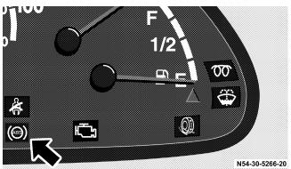
When the key is in position 2 in the ignition lock, the ABS indicator lamp will light up in the instrument cluster. It goes out after about 2 seconds.
