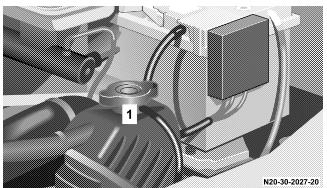
The cooling system is pressurized. Only check the coolant level with the vehicle parking on a level surface and with the engine switched off.
