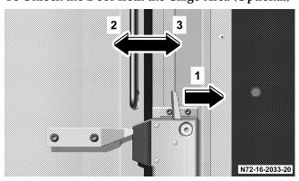
To unlock, press latch in direction (1)
