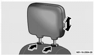
If you need to remove the head restraint, press the catch at the head restraint socket and pull the head restraint up and out.
