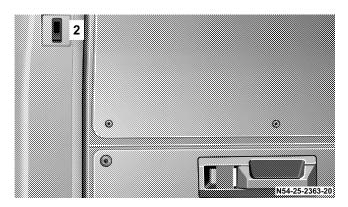
The switch (2) is located in the right rear of the cargo area.
