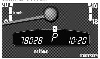
The current selector lever position (1) is indicated in the gear range indicator display. The automatic gear shifting process can be adapted to specific operating conditions using the selector lever.
