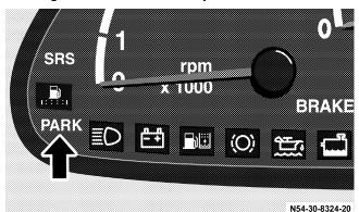
With the key in position 2 in the ignition lock and the parking brake released, the indicator lamp PARK lights up for about 2 seconds.
