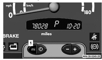
Activate the multi-function indicator. The total distance covered by the vehicle will be shown.
